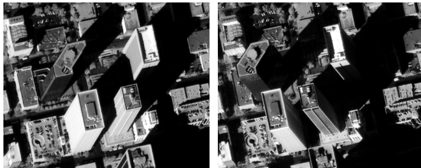
Figure 21: Epipolar Stereo Pair (Courtesy of GeoEye, Inc.)
